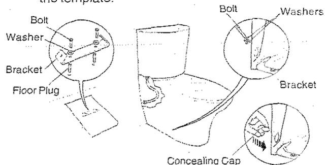
4. Fit the bracket to the floor with the floor plugs, the washers and the bolts.
