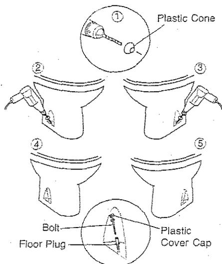
1. Position the WC and install the soil pipe in accordance with the manufacturer's instructions.
