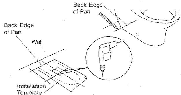
1. Put the WC in position and mark a line along the back of the WC.
