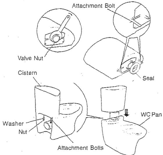
2. Make sure that the valve nut on the base of the cistern is tight.
